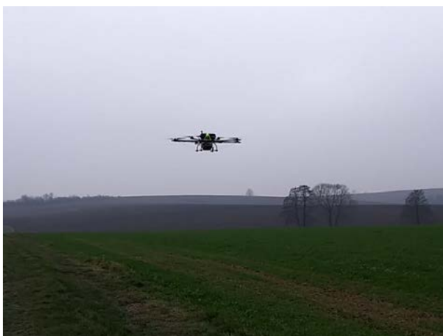
Fig.: 1 The Photo of drone supplied by hybrid power source (battery and hydrogen-air PEMFC stack) during flight.
